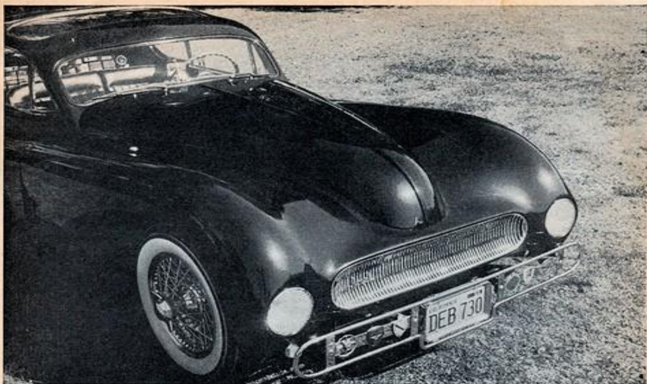
Hood has been lengthened with a hand-formed metal panel merely extending the existing contours. Into the newly shaped grille oval, the owner has installed 65 concave chromed bars, set in a vertical pattern. The shield below the grille has been contoured to the body lines.
