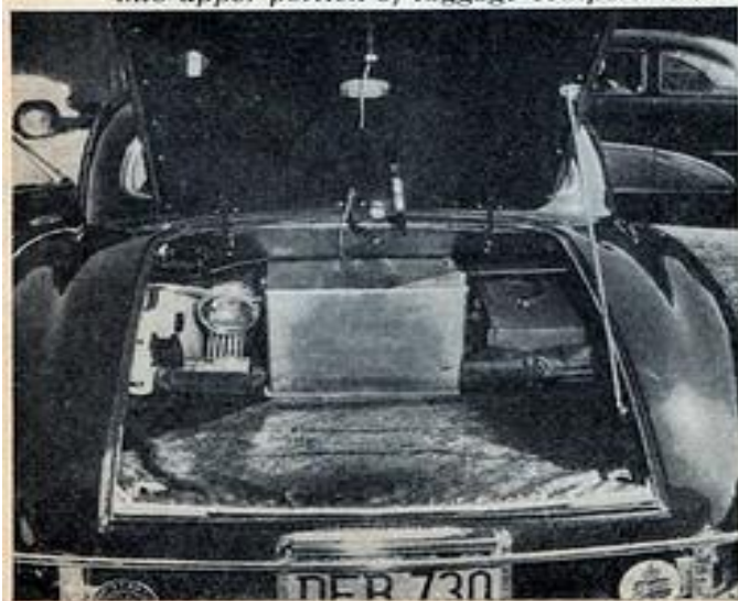
Emergency flares, first-aid kit, trouble lamp, and chrome-plated tool box have been fitted into upper portion of luggage compartment.
